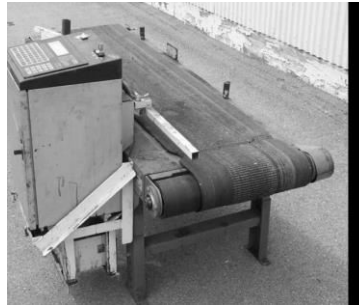
Fig. 2.1.1. A flat belt conveyor with drive control
