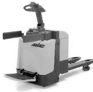
Fig. 3.2.2. Pallet lift truck (battery)
